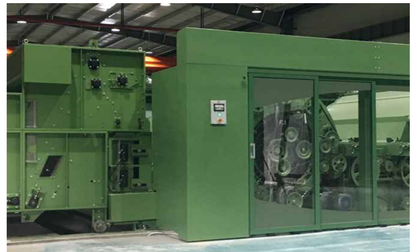
New side doors for Worsted Cards
