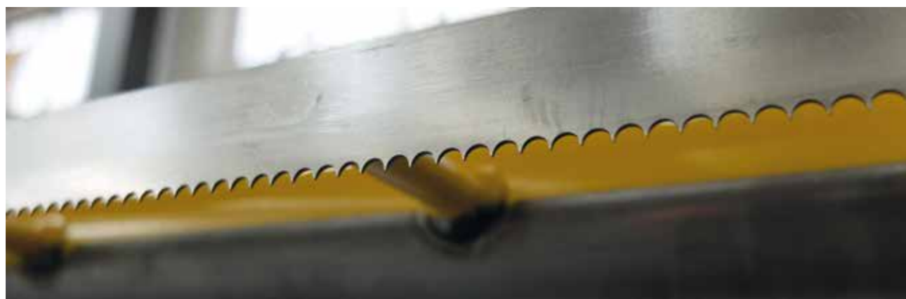
Details of Doffing Combs (Courtesy Officina Meccanica Montenero)
